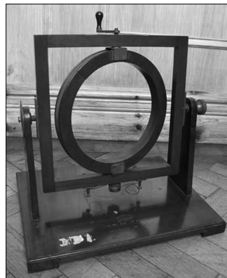
Fig. 14 Earth Inductor by W.G. Pye & Co., Cambridge, England, c. 1910.
