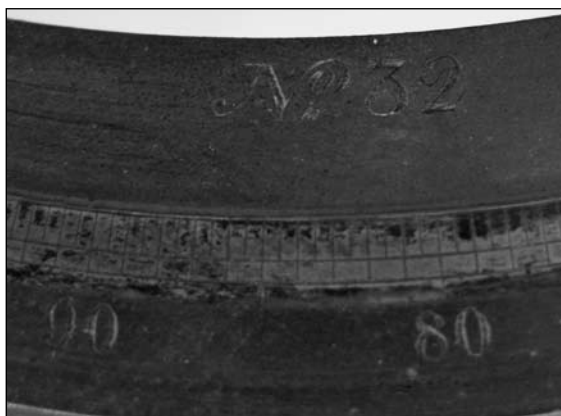
Fig. 6a Dip circle made by Henry Barrow & Co. 26 Oxendon St. London. Height 32 cm; wood frame 17.8 cm square; scale diameter 15 cm; needle length 9 cm. b Detail of serial no. '32'.
