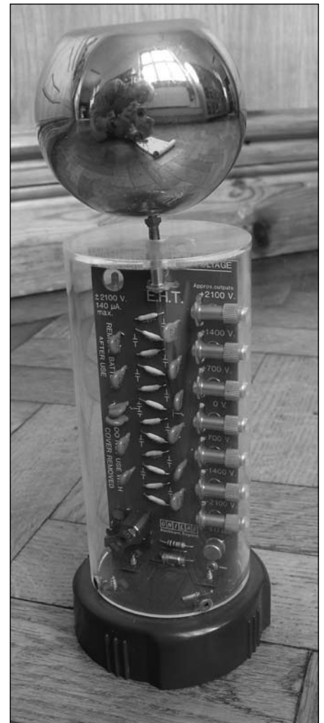
Fig. 16 Cockcroft-Walton high voltage generator using modern semiconductor technology, made in nearby Blackburn, England, by UNILAB. Height, including sphere, 25.5 cm.
