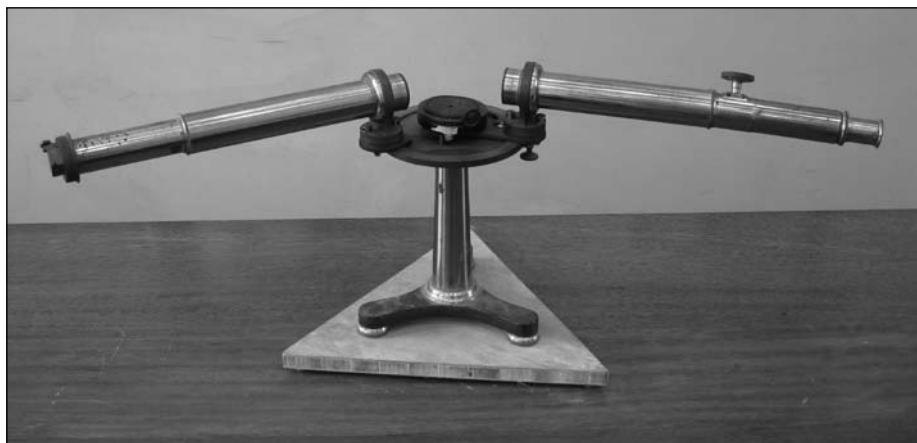
Fig. 10 Spectroscope by 'John Browning 63 Strand London' sans central prism assembly.
